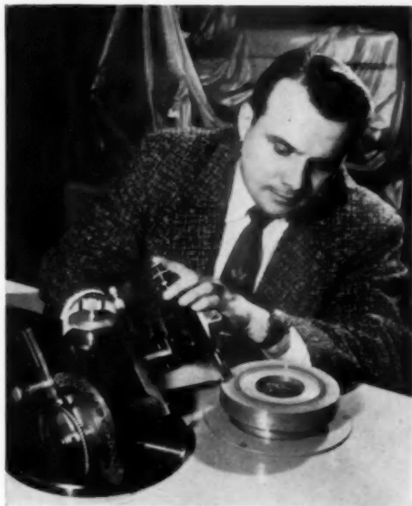
Leo L. Coombs of Park Forest, Ill., forms precision radius tip on tool which he holds against diamond impregnated wheel.
